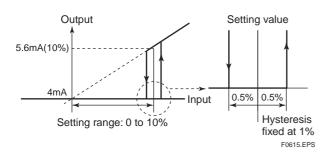
[J11: 4-20mA Low Lmt] Setting of the low limit for current output
